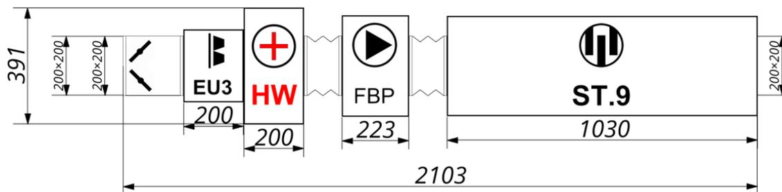
Установка: LM DUCT R 200 /V.1/EG.3/HW.2/G.1/FBP.E22A.2E/G.1/ST.09
