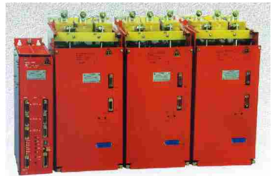
Series ЭТА1-03 thyristor asynchronous electric drives
