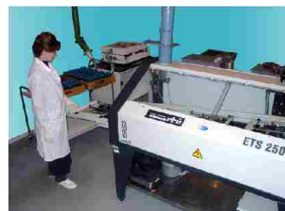
Double-wave soldering machine for PCBs
